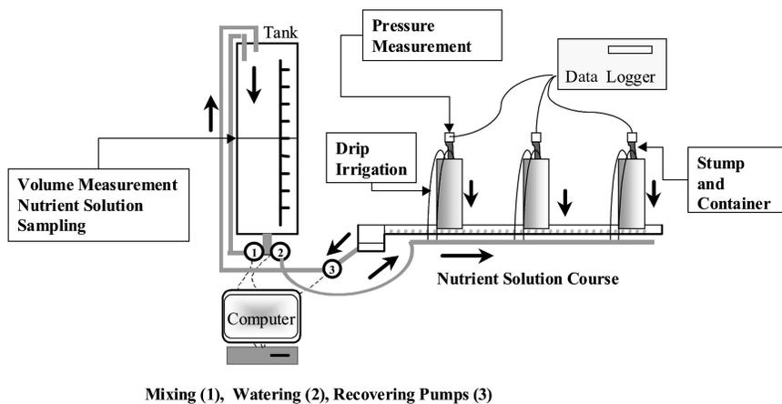
Figure 2. Diagram of drip irrigation system for measuring and recirculating nutrient solutions. Pressure transducers were connected to root stumps while nutrient uptake and soil temperature were monitored.
