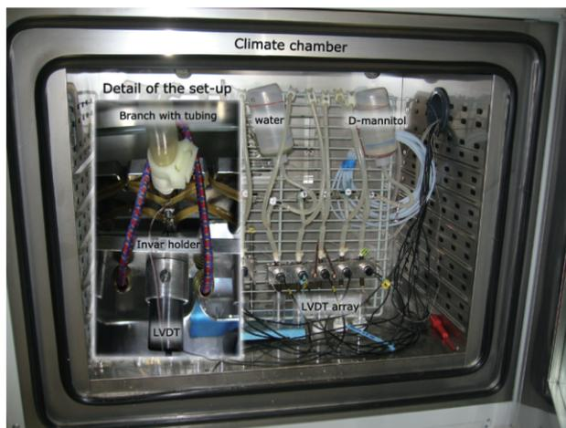
**Figure 1.** Measurement set-up showing the climate chamber and the twig samples mounted in a linear variable displacement transducer (LVDT)-array. The twig samples were fitted to plastic tubing and connected to a reservoir filled with either deionized water or a D-mannitol solution. The inset shows a detail of the mounting of a twig segment.
